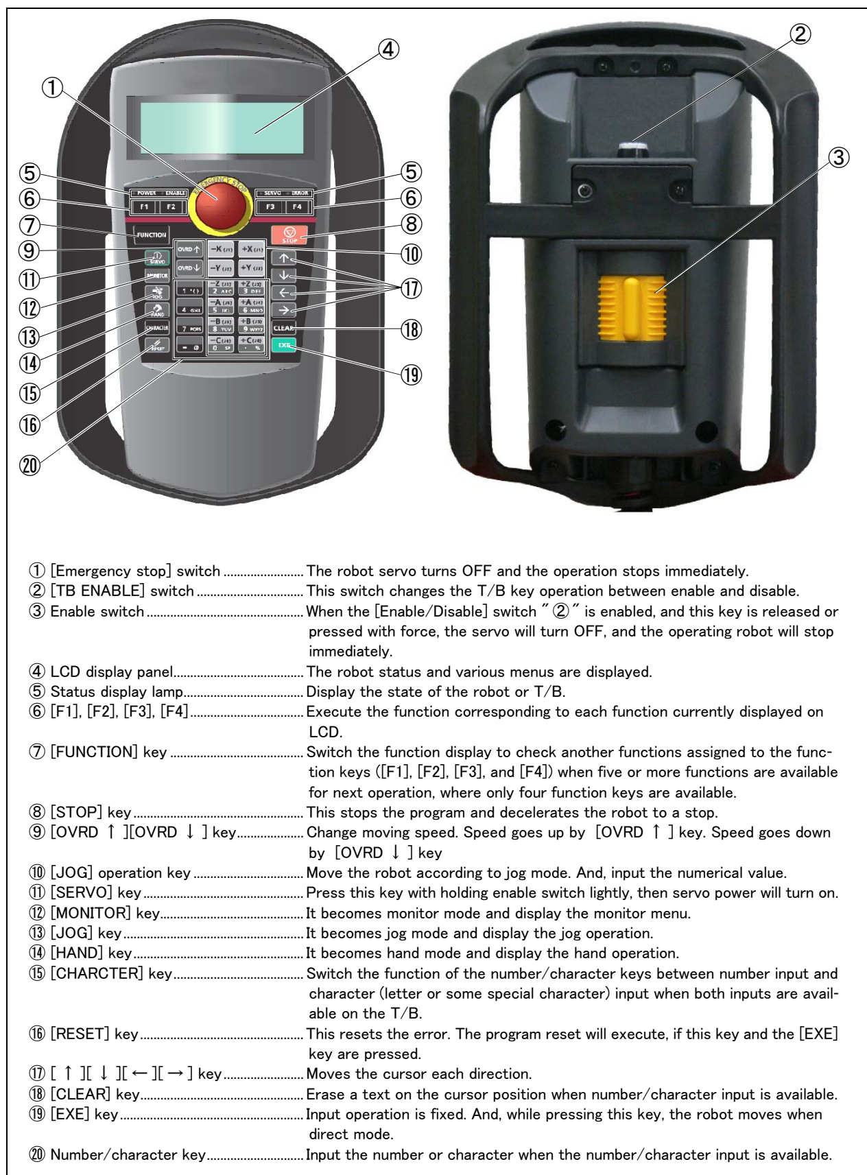
Fig.3-22 : Teaching pendant key layout and main functions
